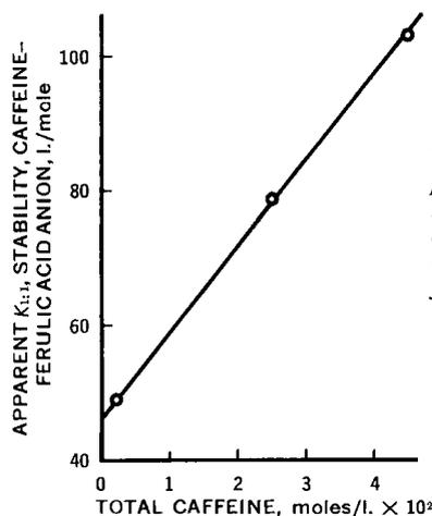
Figure 2—Plot of apparent  $K_{1:1}$  stability constants from partitioning data of the caffeine-ferulic acid anion system as a function of total caffeine concentration at 25°.
