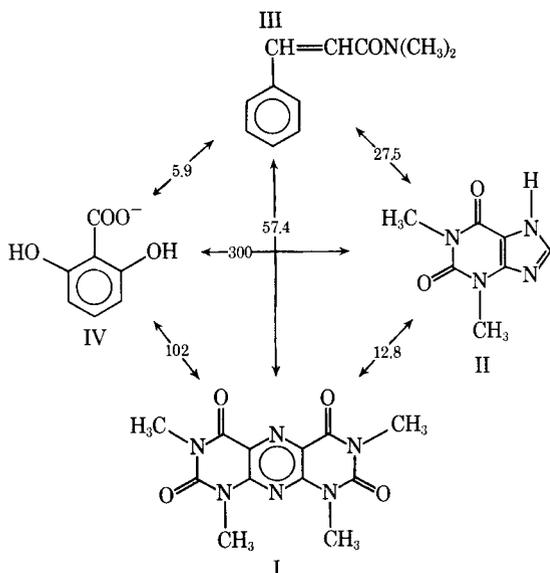
Scheme I—A-B system interactions in water at 25°. The numbers on the arrows represent the 1:1 stability constants for the interacting species. I, TMPPT; II, theophylline; III, *N,N*-dimethylcinnamamide; and IV, 2,6-dihydroxybenzoate
